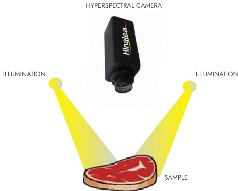
Figure 3: Hyperspectral imaging camera configuration for meat fat and moisture content measurement
