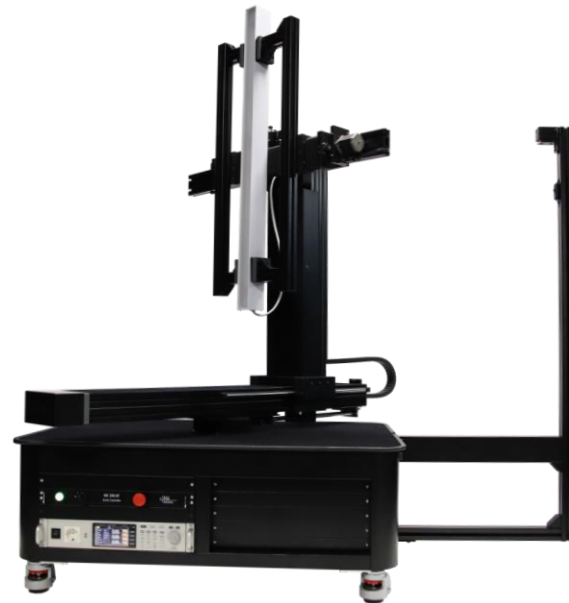
SSL SH Lin-2, 2-handed sample holder for super fast sample mounting.
