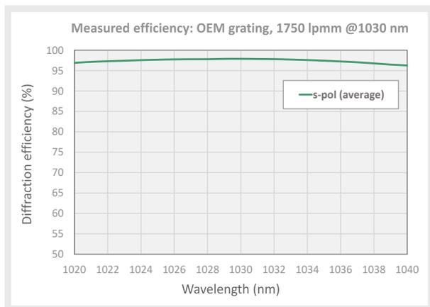
We measure every VPH transmission grating to ensure exceptional 1st order diffraction efficiency. Many other vendors report only theoretical graphs of total diffraction efficiency, which includes diffraction into other orders, and is not truly representative of actual performance.
