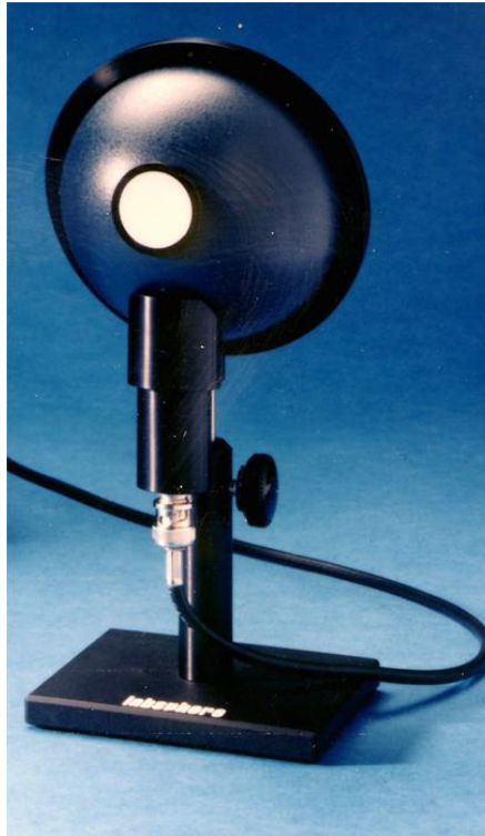
Figure 3: Integrating Sphere for Divergent Source Flux Measurements (courtesy of Labsphere)
