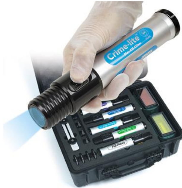
Figure 8: LED-based Torch for Forensic Analysis (courtesy of Mason Vactron)
