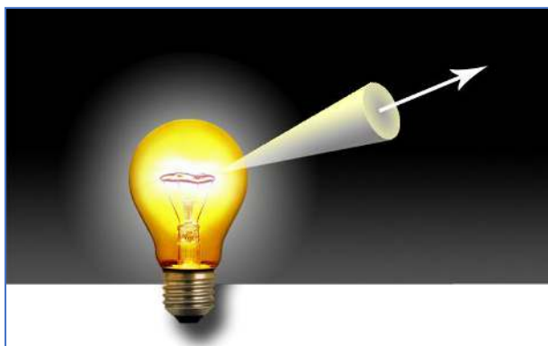
Figure 2: Luminous intensity is the luminous flux emitted in a specified direction per unit of solid angle, units of lumens per steradian, simplified to the candela.
