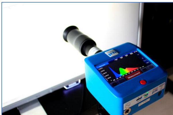
Figure 12: The Spectraval is a portable, hybrid spectroradiometer that measures spectral irradiance, spectral radiance, luminance, illuminance, CCT, CIE chromaticity and colour rendering. It can be used in the photometric laboratory, as well as taken out for site surveys and lighting scheme verification (courtesy of JETI).
