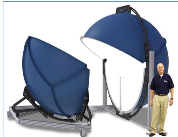
Figure 3: A 3m diameter lamp measurement integrating sphere (courtesy of Labsphere).
