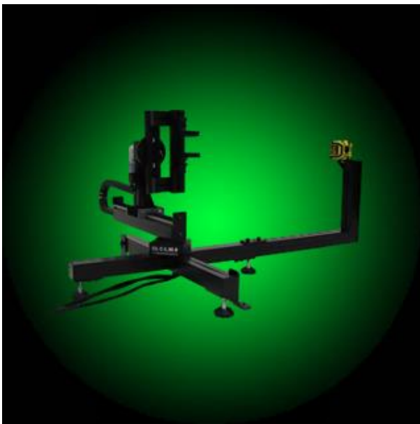
Figure 4: The compact LAMP 30 2-axis motorised goniophotometer from SSL Resource
