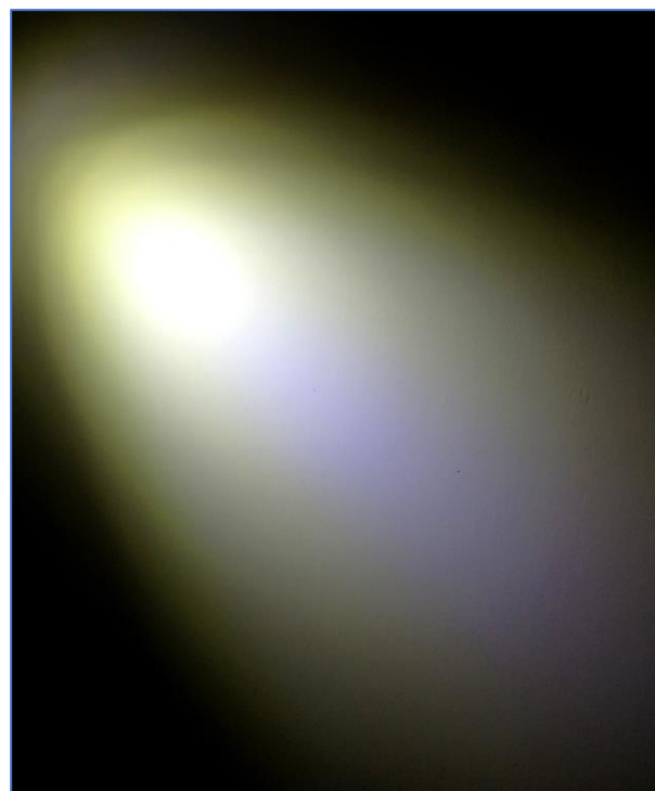
Figure 10: Phosphor white LED colour zoning – note the high CCT (blue tint) in the centre of the beam, surrounded by a yellow-tinted annulus.
