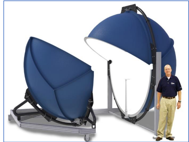
Figure 3: A 3m diameter lamp measurement integrating sphere (courtesy of Labsphere).
