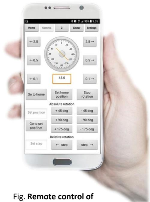
Fig. Remote control of motorized axes through the Android app using Bluetooth
