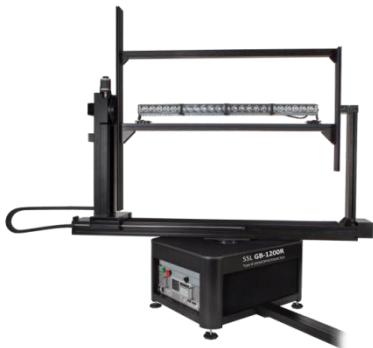
B Type Measurement for Automotive Lights
