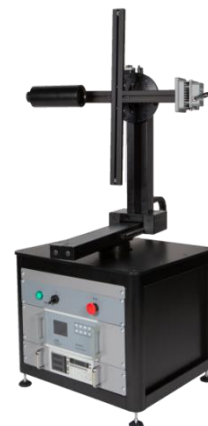
Burning Position Correction Setup for C type (photo: SSL LUMI 90)
