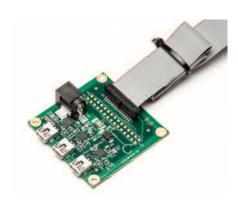
The host adaptor board provides an easy way to connect to the XCD2 main board. A standard header connector has pin to pin connection to HOST connector and has the same signals as the small HOST connector. In additional the board has a power jack connector to supply 5V.
