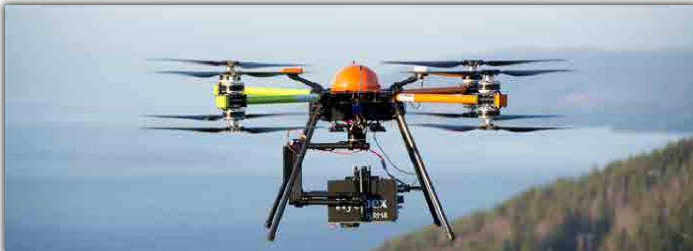
HySpex Mjolnir V-1240 carried by CamFlight FX8HL. NEO offer full integration with CamFlight's robots.
