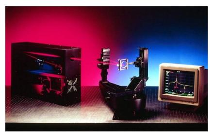
Incident plane scatter measurements with an option for polarization control The CASI™ was developed to provide reflective and transmissive scatter measurements very near the specular beam as well as at high scatter angles. The noise floor is limited by scatter from air molecules, but it also measures right through the specular beam. Measurements can be compared to a "no sample signature scan"
