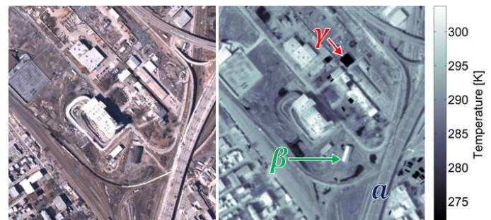
Figure 2 Airborne visible image (left) and broadband infrared temperature map (right) of an industrial area. Selected locations are labeled for further explanations.
