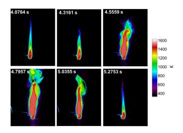
Figure 6 Temperature profile of the plume during the explosion generated by the burning of black powder.
