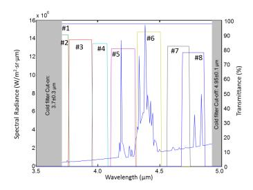
Figure 2 Blue (4.18  $\mu m)$  and red (4.37  $\mu m)$  spikes from the  $CO_2$  overlaid on the transmittance of the 8 spectral filters for better evaluation.
