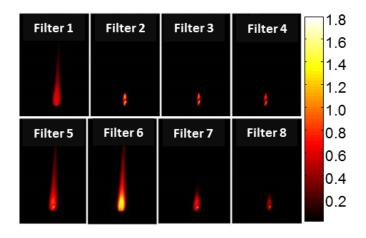
Figure 3 Relative individual spectral channel responses during the candle's combustion.
