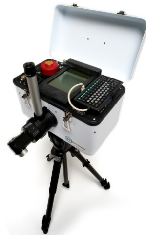
Compact and portable: micro FTIR spectrometer (Model 102)
