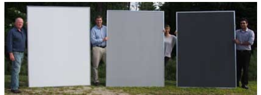
Permaflect Outdoor Reflection Target 94 %, 50 % and 5 % R (Lambertian)
