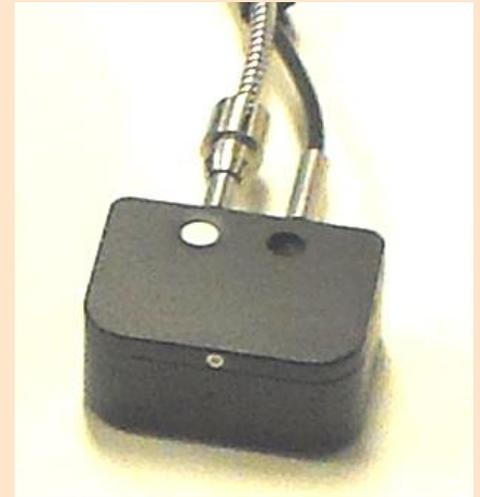
*Each SR-1901PT includes a right angle diffuser with integral phototrigger for easy set up and measurement. TTL electronic triggering is also possible.*
