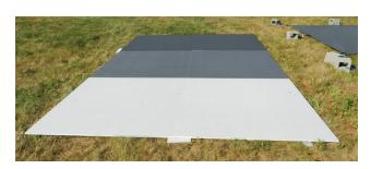
Correct image tonal balance over a broad scale of uniform grey scale reflectances from 5% to 95%
