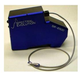
Ultra high resolution, portable spectroradiometer from Spectral Evolution
